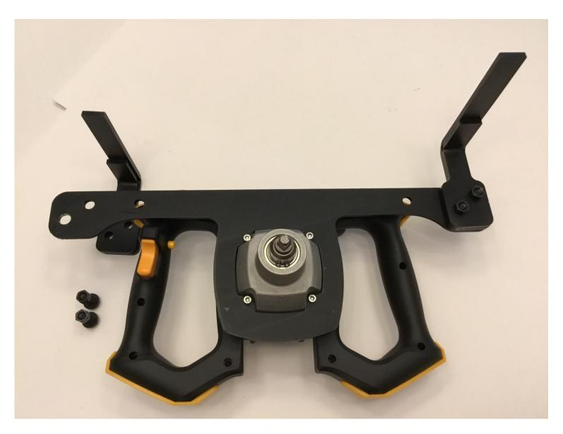
Bolt the pair of support arms, bolts toward the front. Smaller arm goes below the larger one as additional support.
