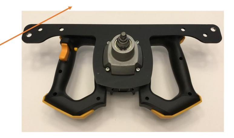
Place SA Plate over the housing and use new screws to bolt it on. Note the direction of the screw holes on plate, must be bottom left to top right.
