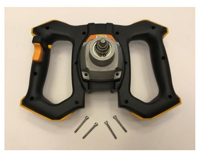
Remove the 4 screws around the gear housing. **DO NOT take the gear housing off.**
